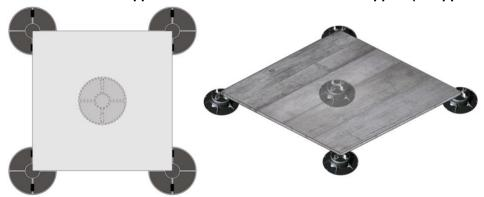
SIZE 60X120 cm: 1 support for each corner, 2 supports 1/3 along the slab and 2 supports half-way along each of the two long sides (4 supports per piece)
