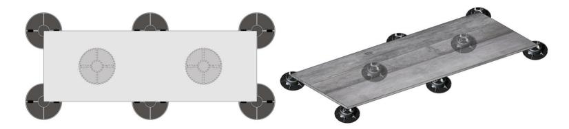
If a greater overlay height is required, Florim recommends glueing a backing plate or safety mesh to the back and additional supports under the slab, as in the attached diagram;
