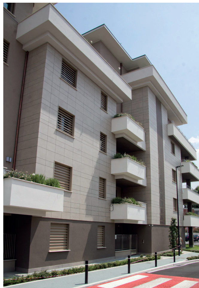
Residential complex- Residential | Novate Milanese (MI) - Italy S5 fixing system - Hidden fixing ventilated façade system for FLORIM tiles maximum size 80x180 cm - 9 mm thickness
