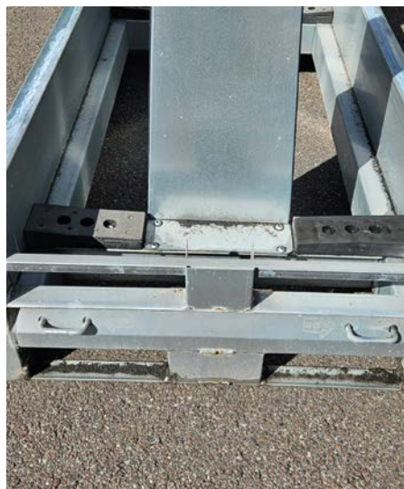
Detail of open hooks for dragging the galvanised A-frame
