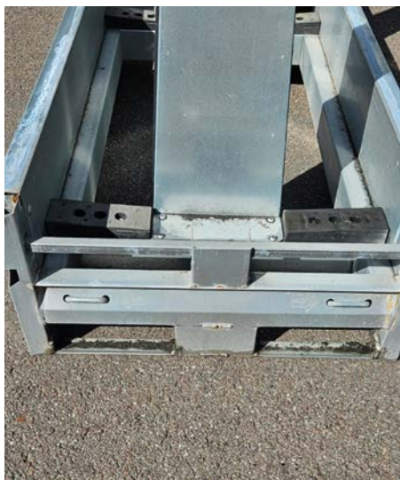
Detail of closed hooks for dragging the galvanised A-frame
